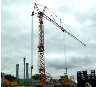
*Figure 3 – Self-erecting tower crane*
