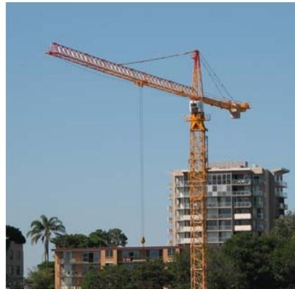
Figure 2 – Hammerhead tower crane
