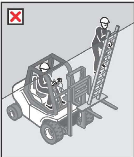
Figure 14: Unacceptable practice with ladder on forklift.
