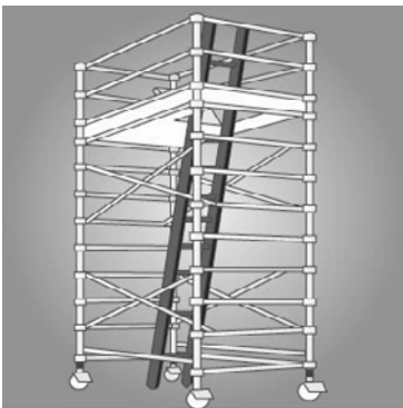
Figure 7: Mobile scaffold with an access ladder and trapdoor to provide the largest possible hazard-free working platform.
